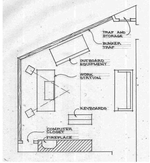
Fig. 3. Concept floor plan for residential production room.
