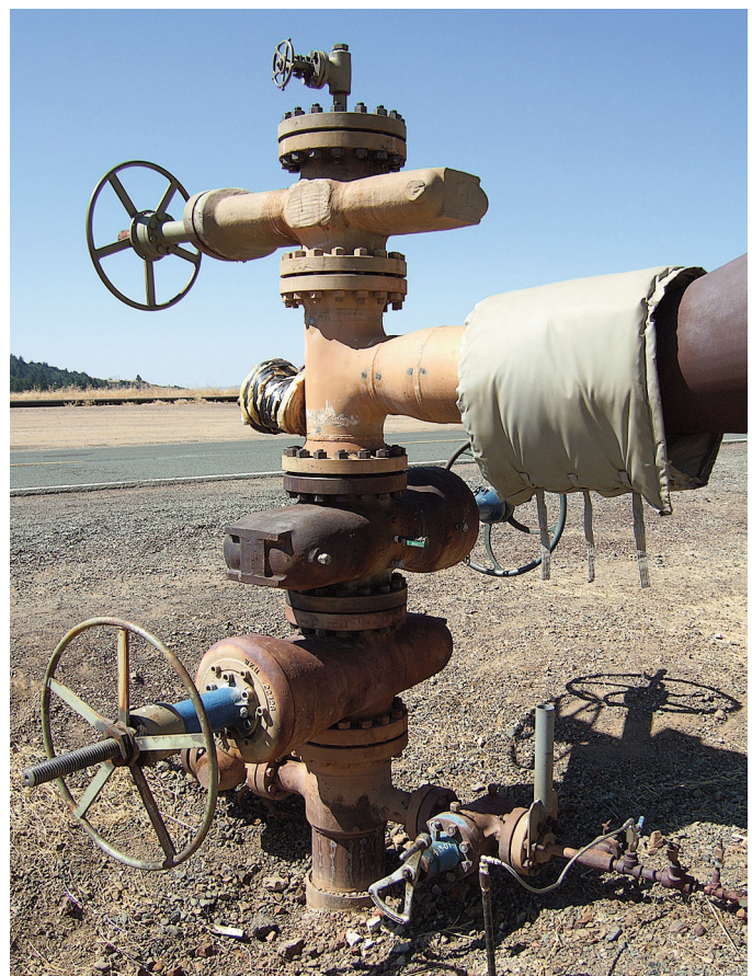
Fig. 1. Steam well at the Geysers geothermal field near Calistoga. (Courtesy http://www.flickr.com/photos/kqedquest/1544212039/ ).
